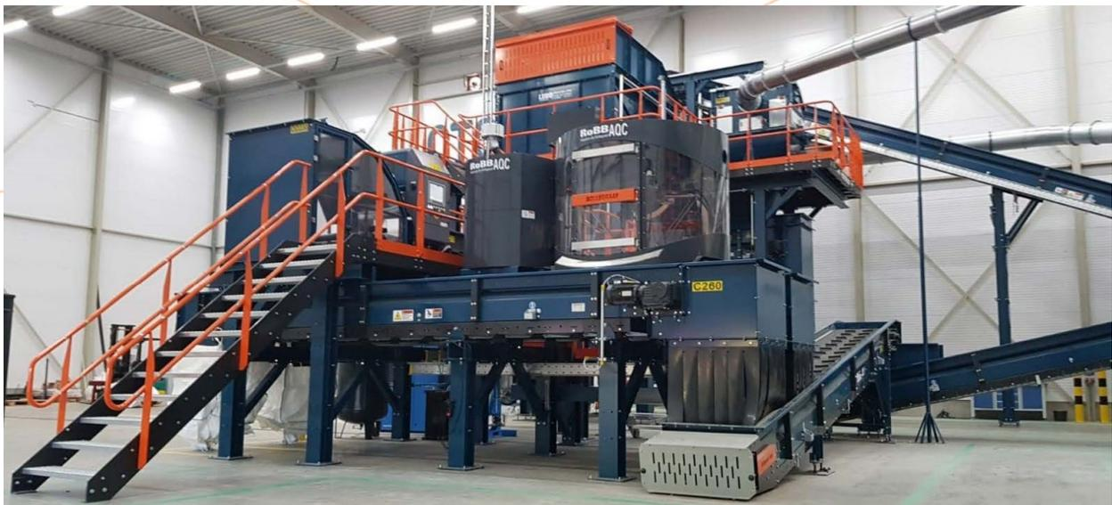
Bollegraaf Recycling Solutions was honored by the trust placed in 2020 by the NTCP for the design, production and installation of a unique modular sorting facility aiming at testing and improving the recyclability of plastics from household waste.
