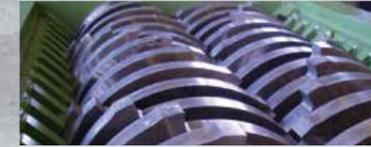
*Crude shredding shear blades / Large teeth (35 mm) are used for rough shredding, whereby capacity can be increased (to a maximum of approx. 6,000 kg/h) by defining the header side of the shear blades at an angle. This increases the grip on the material that is to be shredded.*
