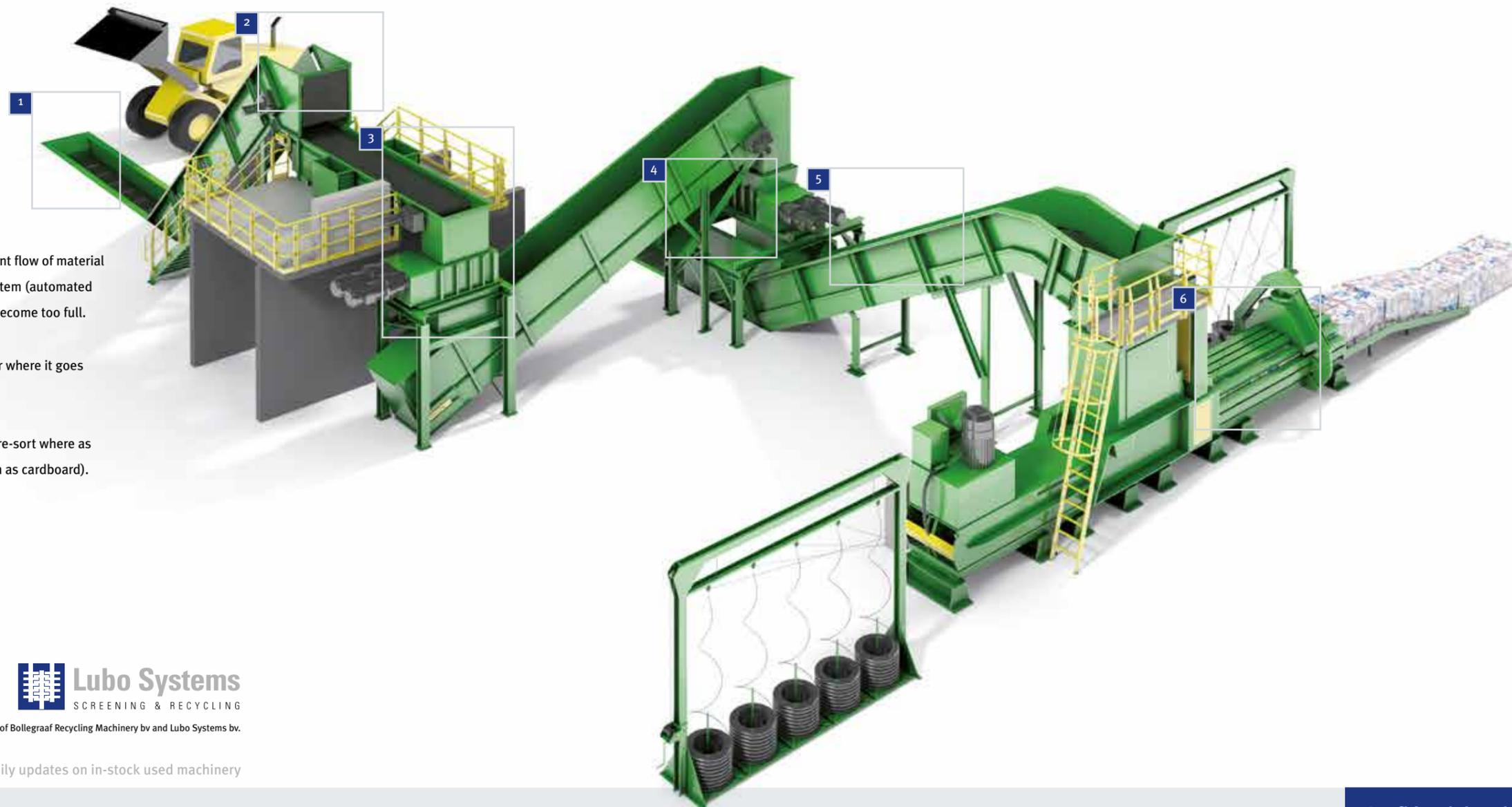
**5** Next the material goes back on a conveyor to the second shredder (fine shred). The ferrous metals are removed using a belt magnet. There is also a bunker (feeder belt) here that gives the system additional flexibility if one shred phase can be omitted (for example, non-confidential information).
