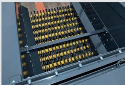
The coarse fraction is separated in the first phase. This gives the Antares a high capacity level.
