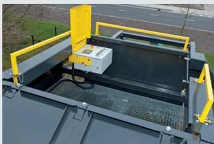
The position of the control panel gives you an optimum view of the screen deck and the output stream.
