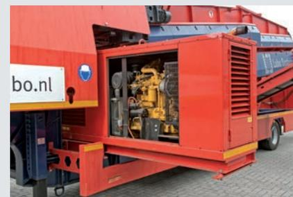
The open structure of the machine ensures that the parts can easily be accessed for maintenance work.
